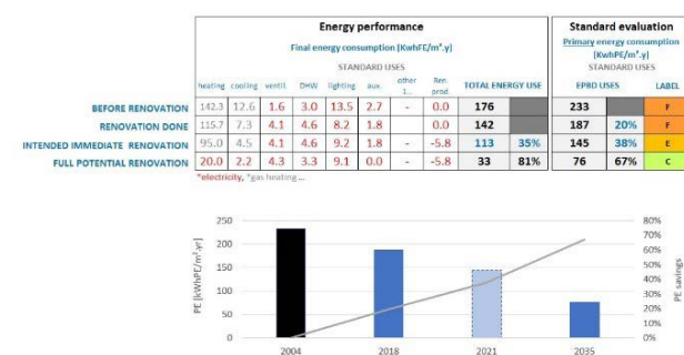
Figure 6. Example of connection of energy ratings with the RenoMap, thermal environment and financial valuation (pilot building Maly trh 2/A, Bratislava).
